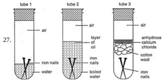
Test tube 1: Iron nails would get rusted that is corroded as they are exposed to moisture and air.
